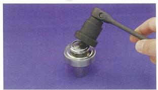
Use a tightening tool made especially for **FINE U-NUT**.
