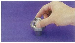
Manually screw the nut on until the friction ring touches the tip of the threaded portion of the shaft.
