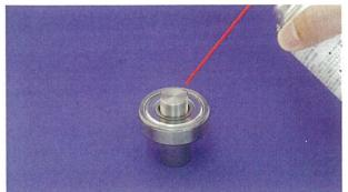
Position nut on shaft. Apply lubricant after checking that the tip of the thread portion of the shaft has a chamfer that is equivalent to the distance of 1 pitch. When the shaft has low hardness, use lubricant with especially high lubricating properties.
