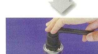
Press down on the axis portion of the ratchet handle and tighten by lightly turning the ratchet.
